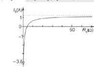
The graph of the function is a hyperbola. Its special points are: at  $R_x = 0 I_3 = -3.8 A$ ; at  $R_x$ ; =  $4I_3 = 0$ ; at  $R_x = 32\Omega$   $I_3 = 1A$ ; If  $R_x \to \infty$ ,  $I_3$  tends to 19/16 = 1.1875A.
