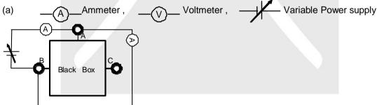
(b) See graphs for the calculations of slopes.  $R_{AB} = 0.98 \text{ k}\Omega$ ,  $R_{BC} = 4.60 \text{ k}\Omega$ ,  $R_{CA} = 5.67 \text{ k}\Omega$
